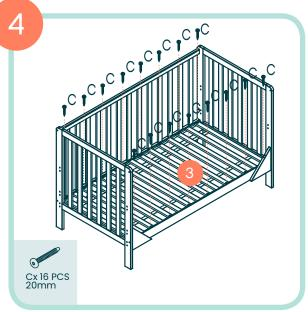
Assemble the mattress base (3) using 16 x C bolts
