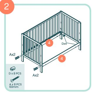
Assemble the two ends (1) with one of the cot sides (2) using 4 x A bolts and 4 x D unts
