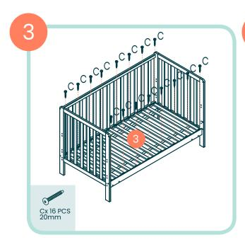
Assemble mattress base (3 )using 16 x C bolts
