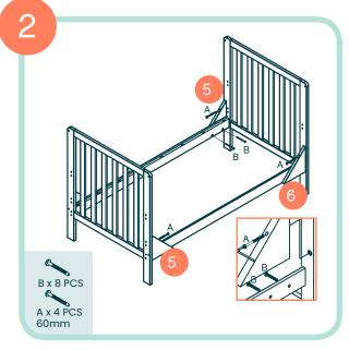
Assemble the two ends (1) with the two mattress support rails (4) using 8 x A bolts and 8 x D nuts
