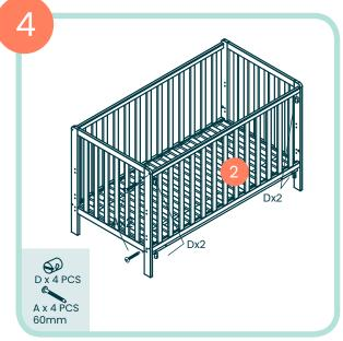
Assemble the two ends (1) with the other cot side (2 ) using 4 X A bolts and 4 x D nuts
