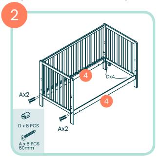
Assemble the two ends (1) with one of the cot sides (2) using 4 x A bolts and 4 x D nuts
