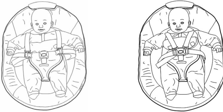
Place the child in the seat as shown in figure. Insert the left and right sets of straps into the restraint latch. A "click" will indicate the correct fastening. Adjust the harness to fit the height of your child, using the restraint fits. The harness should fit snugly but not too tightly. The right regulation should allow to insert a finger.
