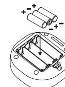
2. Open battery door compartment and insert 3 new AA (1.5V) Alkaline batteries. Be sure to insert with correct polarity.
