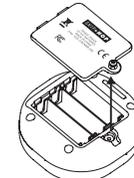
1. Loosen the battery door screw using a Philips head screwdriver.
