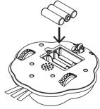
Open battery door compartment and insert three new AA (1.5V) Alkaline batteries. Be sure to insert with correct polarity.
