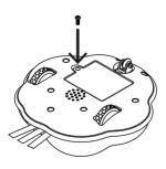
3. Position the battery door securely back into place and tighten with a screwdriver.
