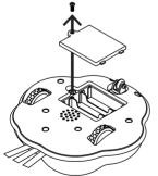
1. Loosen the battery door screw using a Philips head screwdriver.
