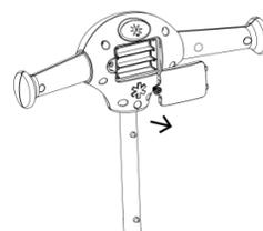
1. Loosen the battery door screw using a Philips head screwdriver.
