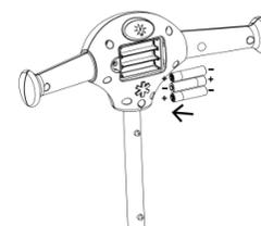
2. Open battery door compartment and insert three new AAA (1.5V) Alkaline batteries. Be sure to insert with correct polarity.
