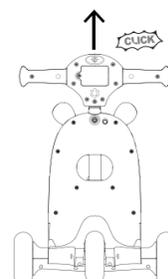
2. Raise handle by pressing screwdriver into LEFT adjuster hole and pulling to release the upper button. Release the screwdriver and pull until the lower button clicks into place.
