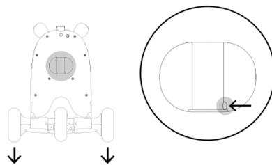
3. Re-insert front wheels with the "locator" in the BACK. Check the window to make sure the metal button is visible on the LEFT side.
