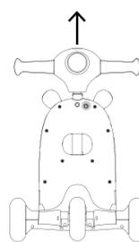
2. Remove front wheels by pressing metal button in the window and pulling the wheels all the way out.
