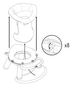
**3.** Turn seat over and insert seat cover through the middle of the seat. Attach all 8 clips on the cover to the seat.
